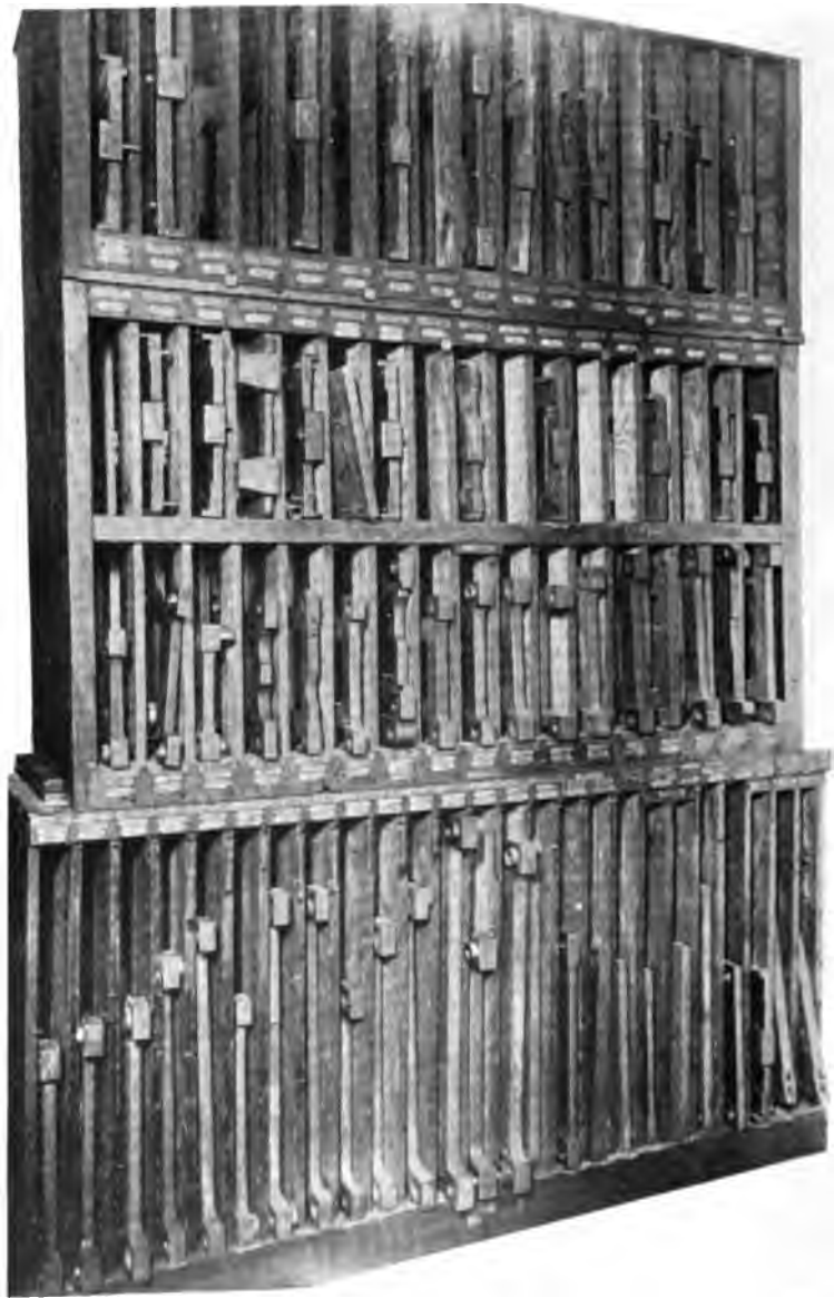
FIG. 5. — Rack with compartments for jigs and templates.
